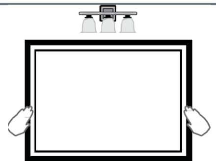
Note: If you accidentally install the frame in an undesired location, place something thin and sturdy (like fishing line) between the frame and the mirror and wiggle downwards - breaking through the adhesive.
