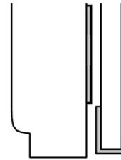
If a mirror has been installed with a j-channel at the bottom, make sure no tape comes in contact with j-channel. If it does, simply remove that section of adhesive so that the channel and the adhesive can lay side-by-side behind the frame.
