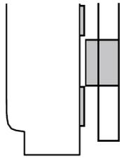
If a mirror has been installed with plastic mirror clips, replace them one at a time with flat metal offset mirror clips. Remove the double back tape from the area where the offset clips contact the back of the Add A Frame®.
