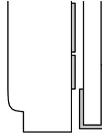
If a mirror has been installed with a j-channel at the bottom, make sure no tape comes in contact with the j-channel.
