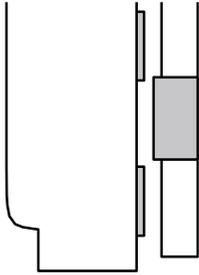
If a mirror has been installed with plastic mirror clips, replace them one at a time with flat metal offset mirror clips. Remove the double back tape from the area where the offset clips contact the back of the Add A Frame.
