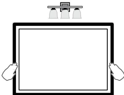
Remove the backing from the tape. Be careful not to touch to the mirror yet. Align the Add A Frame and gently press onto the mirror.
